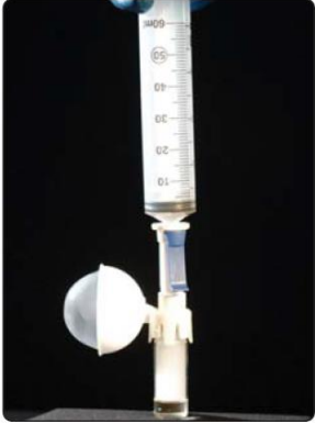
Figure 1. PhaSeal with no release of titanium smoke.
