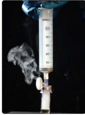
Figure 3. Alaris Smart Site with release of titanium smoke.
