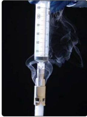
Figure 2. OnGuard Tevadaptor with release of titanium smoke.
